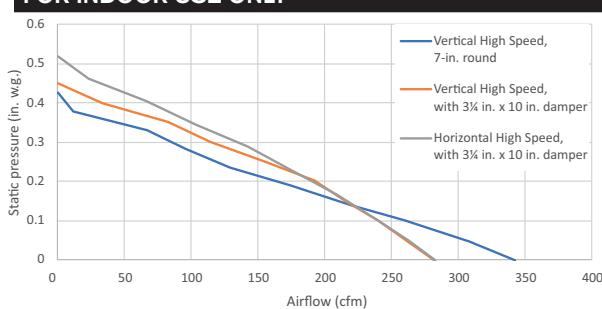
HVI-2100 CERTIFIED RATINGS comply with new testing technologies and procedures prescribed by the Home Ventilating Institute, for off-the-shelf products, as they are available to consumers. Product performance is rated at 0.1 in. static pressure, based on tests conducted in AMCA's state-of-the-art test laboratory. Sones are a measure of humanly-perceived loudness, based on laboratory measurements.
