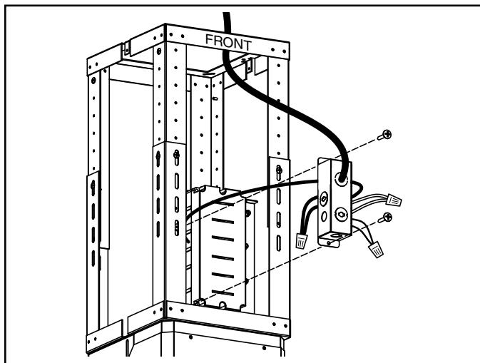
1. Remove wiring cover and connect house wiring to hood wiring
