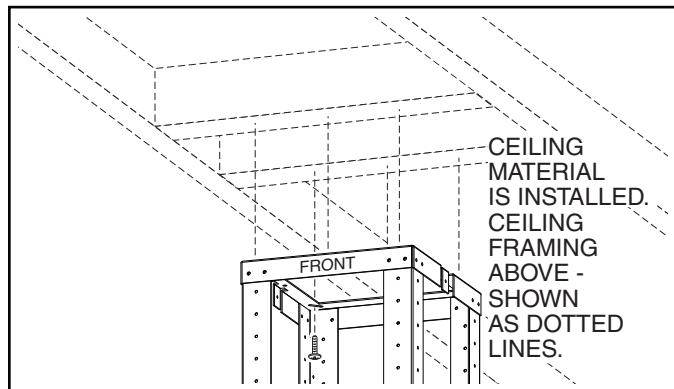
2. After ceiling surface is finished, align frame assembly to ceiling framing, and attach to ceiling framing with (6) 4 mm x 38 mm screws. Tighten securely, making sure that the upper frame bracket is tight against the ceiling.
