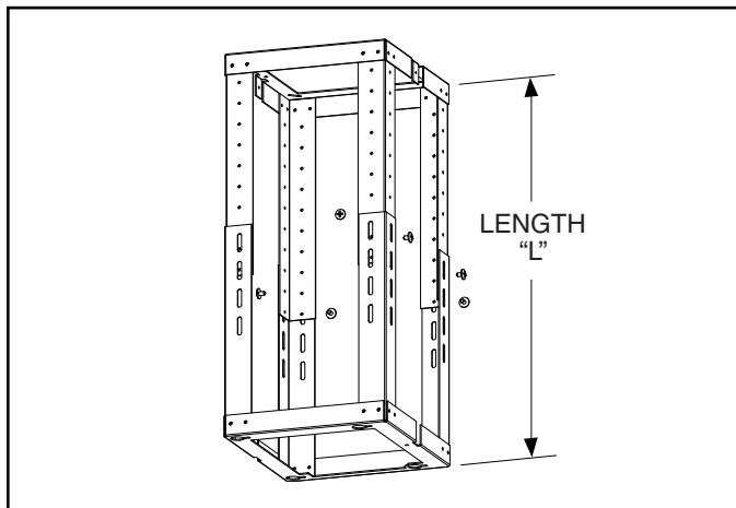
1. Determine length "L" of frame assembly based upon desired installation height (see chart below.) To adjust frame assembly height, remove (8) screws, slide upper frame assembly to required height, replace screws and tighten securely.
