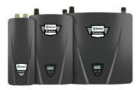
ferent models ranging from 2.4kW to 32kW and a Uniform Energy Factor up to 0.93. The units are available in a variety of voltage options: 120V, 208V, 240V and 277V. All models feature true Dry Fire Protection-the element will only turn on when the chamber is full of water-as well as Scale Reduction Technology. | **Circle 101 on inquiry card**
