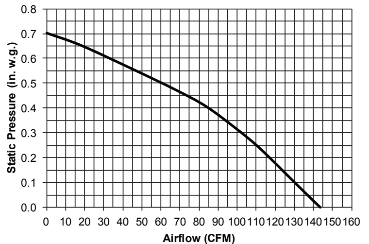
MODEL QT140LE - 4" DUCT
