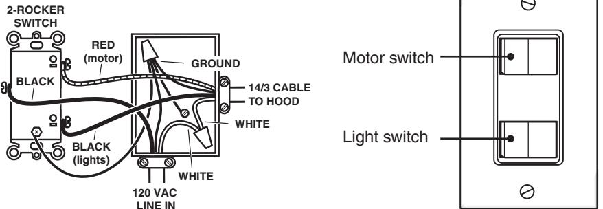
**NOTE:** Allow enough length of 14/3 cable to perform the RED wire connection in the hood nose.
